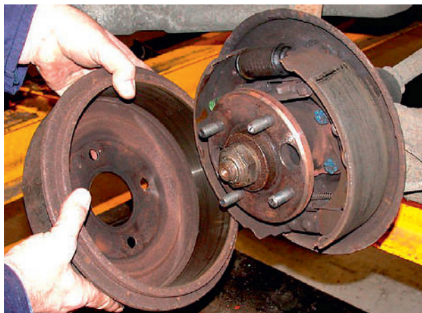
Figure 4.95 Brake drum being removed
